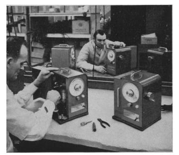
**Top precision** of semi-automatic Fisher Tensiomat\* is assured by careful craftsmanship that's applied to each instrument Fisher <u>makes</u>. Easy-to-use Tensiomat quickly measures both surface and interfacial tension of liquids. #Fisher Scientific Company Trademark
