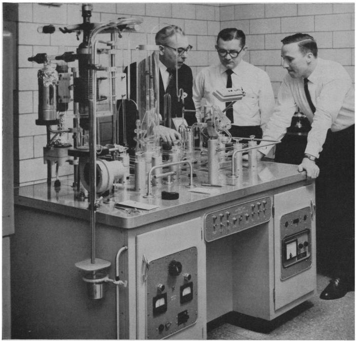
**Exact measurement** of hydrogen, oxygen and nitrogen in metals is made in a few minutes with the Serfass Gas Analyzer. It determines traces of these gases down to 0.1 part per million ... can be used both for vacuum fusion and hot extraction. Here, a Fisher Technical Specialist (left) discusses a problem with the Assistant Chemist and Chief Chemist of Vanadium-Alloys Steel Co.
