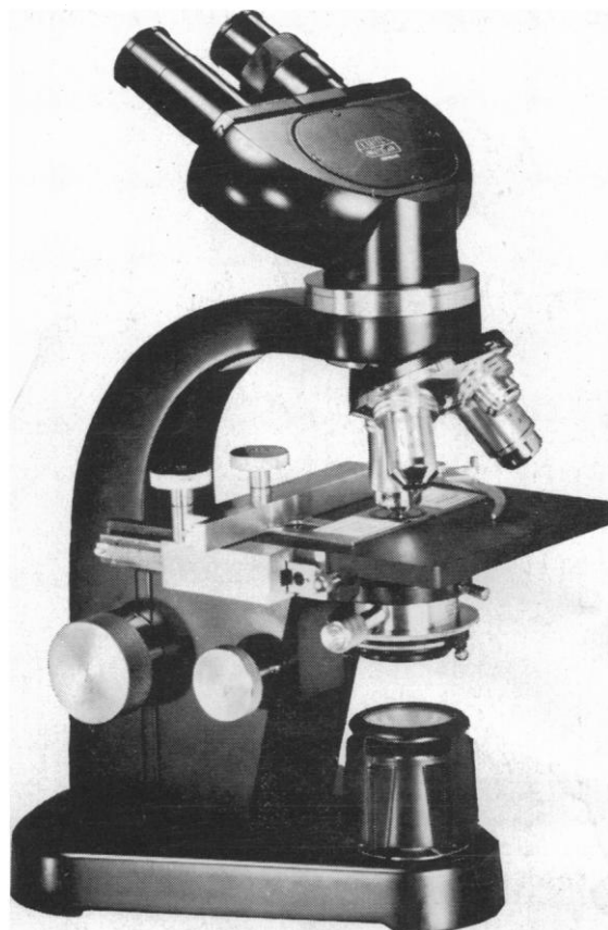
BINOCULAR MEDICAL AND LABORATORY MICROSCOPE SM. Equipped with inclined binocular body; mechanical stage; two-lens condenser with swing-out upper element and iris diaphragm; quadruple nosepiece; mirror and fork. Optical outfit with achromats 3.5x, 10x, and 45x and 100x oil immersion with spring-loaded mounts plus 10x eyepieces.
