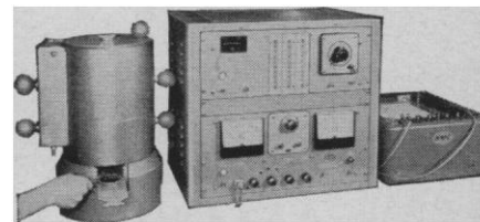
A complete gamma spectrometer system NMC model GSS-1 ($4,180 fob, Indianapolis)
