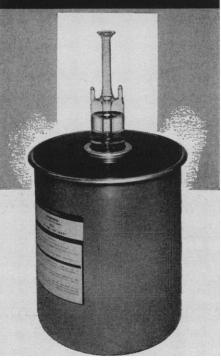
EQUIPHASE Triple-Point-of-Water Cell establishes a reference temperature of 0.01°C with guaranteed accuracy of 0.0005°C. Unaffected by atmospheric pressure, contamination-free, easy and convenient to use. Just 17" high, 8" diameter.
