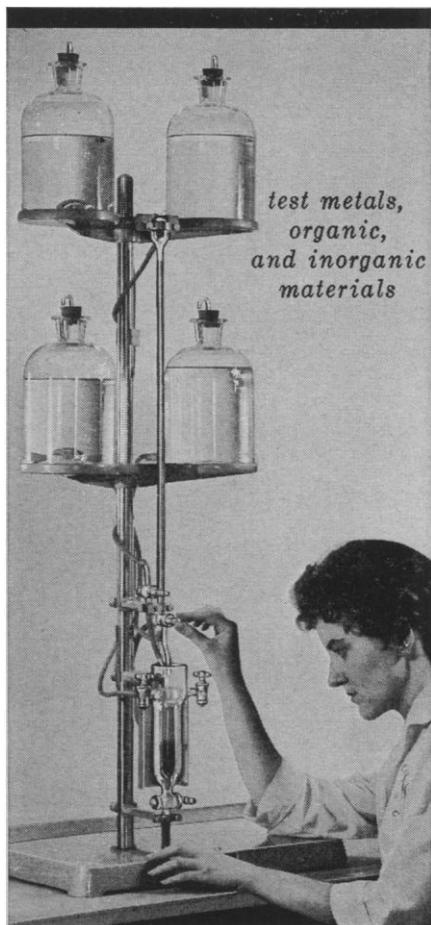
The Dietert-Detroit Sulfur Determinator features an extremely simple direct-reading burette. No involved measuring or computing. Provides fast accurate analysis of sulfur content in a great variety of materials. Low cost, durable, easily maintained. Used in laboratories and institutions for over 22 years.
