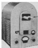
(Left) Dietert-Detroit No. 3420 Varitemp Combustion Furnace for use in conjunction with the Sulfur Determinator (Carbon Determinators also available).
