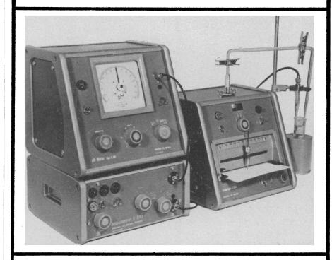
Fully automatic recording of titrant volume as a function of pH (mV), and only new Metrohm equipment has these
