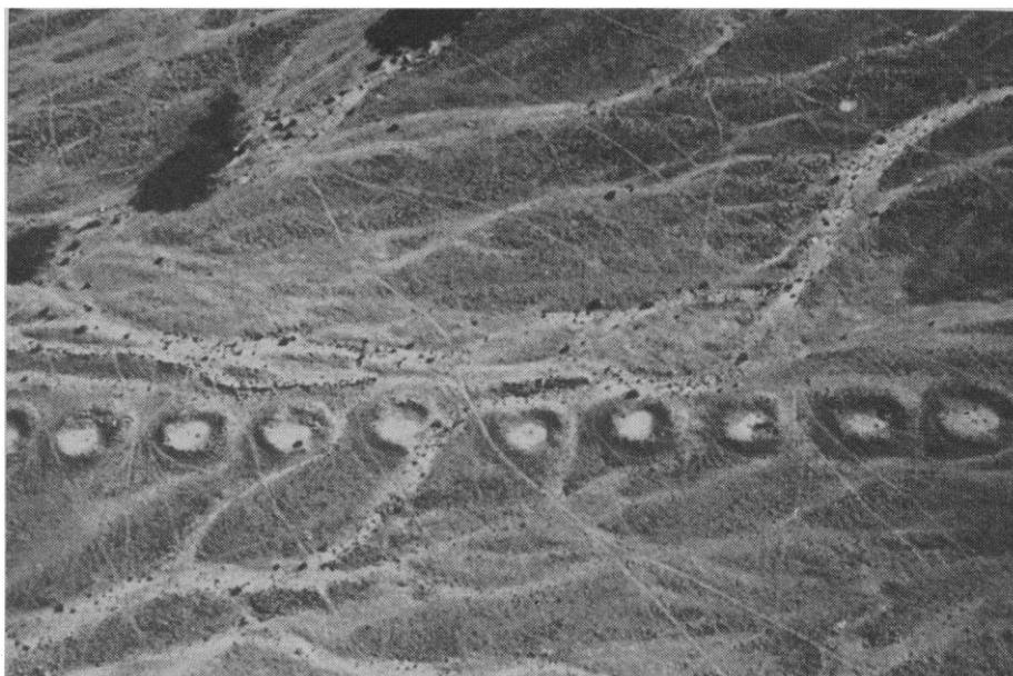
Fig. 12. An oblique aerial photograph of a chain-well system near Ein Ghadian.
