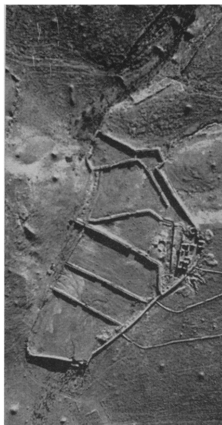
Fig. 14. An aerial photograph of the reconstructed Shvithah farm. Note one branch of one runoff conduit entering the farmhouse, bringing water to an underground cistern.
