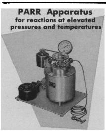
The PARR Series 4500 pressure reactor has innumerable uses for catalytic hydrogenation, alkylation, hydrolysis, polymerization, sulfonation and other applications requiring pressures to 1000 psig. and temperatures to 350 C.
