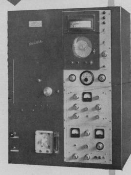
The new Burrell Kromo-Tog Model K-7 is designed for the most accurate chromatographic analysis possible. Its thermionic emission ionization detector has greatly increased sensitivity, speeds analysis and permits use of small diameter columns and smaller samples. It is the only method that will analyze both organic and inorganic compounds as well as fixed or permanent gases.
