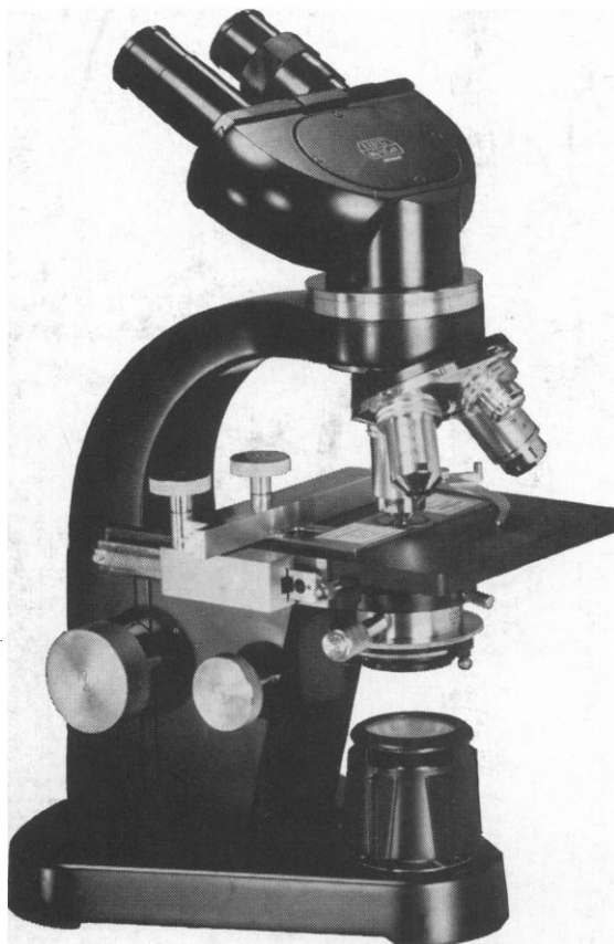
BINOCULAR MEDICAL AND LABORATORY MICROSCOPE SM. Equipped with inclined binocular body; mechanical stage; two-lens condenser with swing-out upper element and iris diaphragm; quadruple nosepiece; mirror and fork. Optical outfit with achromats 3.5x, 10x, and 45x and 100x oil immersion with spring-loaded mounts plus 10x eyepieces.
