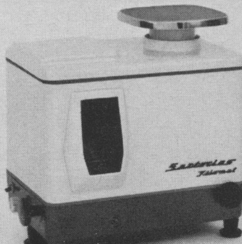
KILOMAT—a new series of fully automatic precision balances for gross weighings in plant and laboratory.
