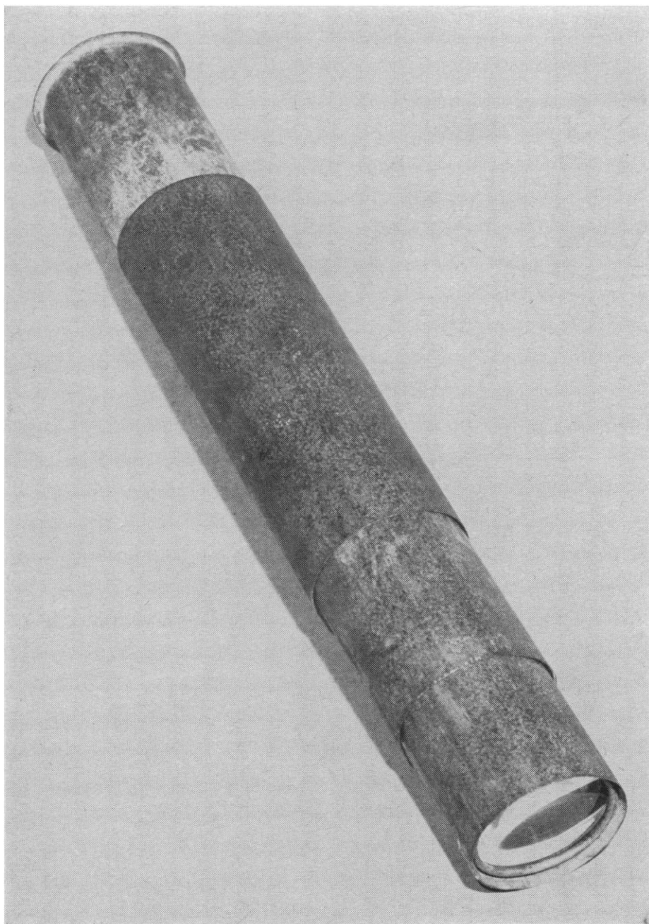
Replica of Hans and Zacharias Janssen's compound microscope, copied from the original. [Armed Forces Institute of Pathology, picture No. 53-662-1]
