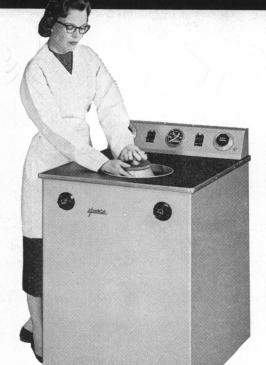
The standard equipment for doing density gradient work is the Model L Preparative Ultracentrifuge (left) and SW-39 Swinging Bucket Rotor (above). The rotor operates at speeds to 39,000 rpm, generating 173,000 g at the outer tube edge.
