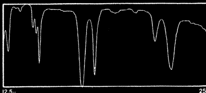
KBr Model 137. Scans from 12.5\mu to 25\mu in 6.5 minutes; provides data impossible or difficult to obtain at shorter wavelengths.
