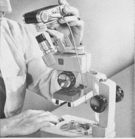
SWING the mounted 35mm Graflex Stereocamera into position over eyepieces. Designed exclusively for Cycloptic, special compensating prisms in adapter unit render camera parfocal with microscopes' optical system. Set camera for bulb exposure. No further adjustment is necessary.
