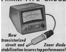
Wide range, fine calibrations, and easy reading are attained with its wide scale, illuminated meter movement and dual reading scale, (.1 microns Hg. to 5000 microns Hg.). It is self-calibrating. A new transistorized circuit insures long, trouble-free use and Zener diode stabilization helps to insure accuracy to better than .1%. The gauge is shock resistant to 8 g.'s and is made of strong polyester, shockproof case and mount. 115 V.—50-60 cycle operation. 6" wide x 6½" high x 8½" deep. Only \$149
