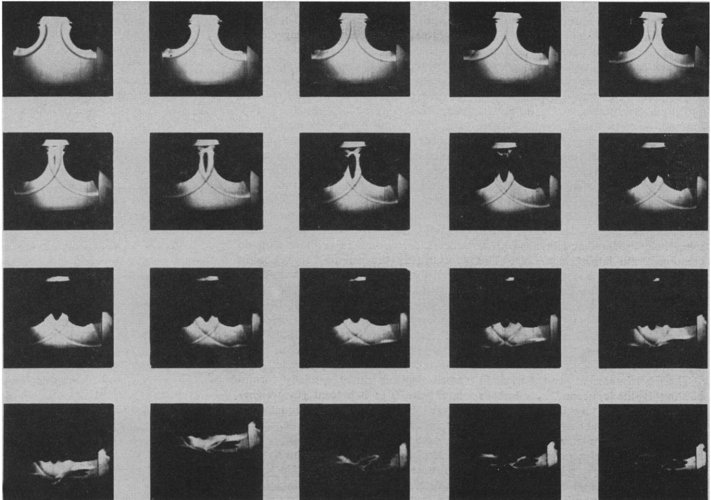
Fig. 9. Megaframe-per-second photographs of shock waves and fragmentation patterns in back-lighted Lucite.
