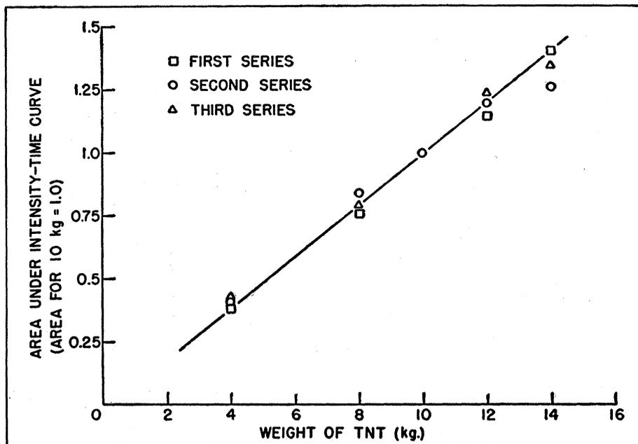
Fig. 5. Measured relative seismic energies for fine TNT at 0.9 gram per cubic centimeter.
