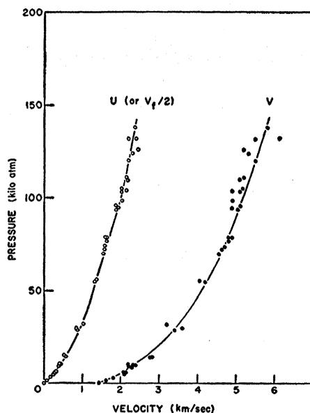
Fig. 7. Calibration  $p(V)$  curves for water shock waves (36).
