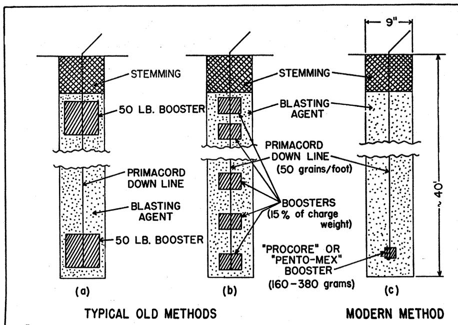
Fig. 1. Diagrams of loaded well-drill holes.
