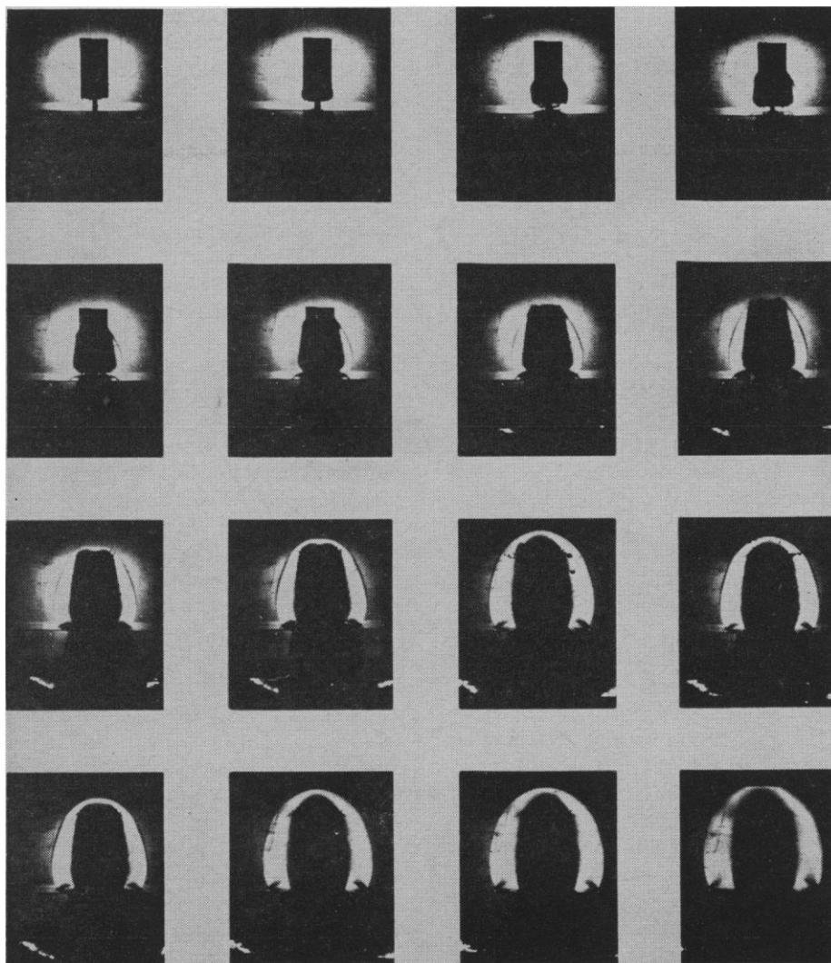
Fig. 8. Megaframe-per-second photographs of a cylindrical charge detonated in the back-lighted aquarium.
