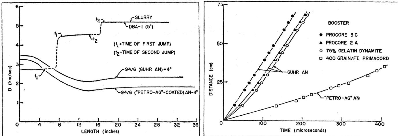
Fig. 3 (left). Velocity transients in unconfined prills and oil (94/6) and slurry with "Pento-Mex" boosters. Fig. 4 (right). Distance-time records in prills and oil (94/6) with different boosters.
