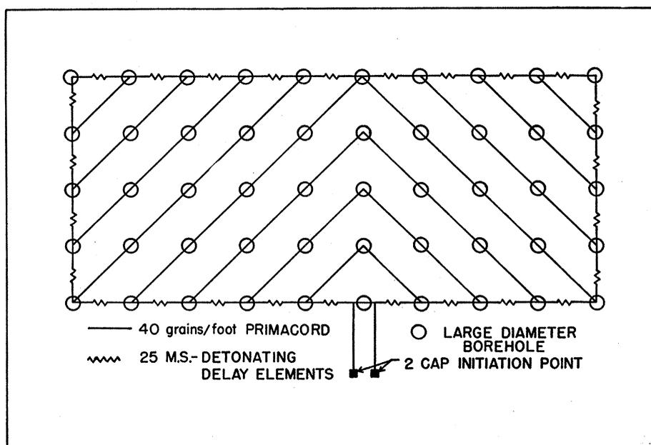
Fig. 2. Typical patterns in multiple-hole blasting.
