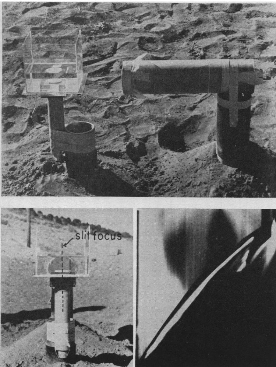
Fig. 6. The aquarium. (Top) Side view; light bomb at right; charge protruding into the aquarium. (Bottom left) End view. (Bottom right) Typical streak camera (time-distance) trace of shock wave in water.
