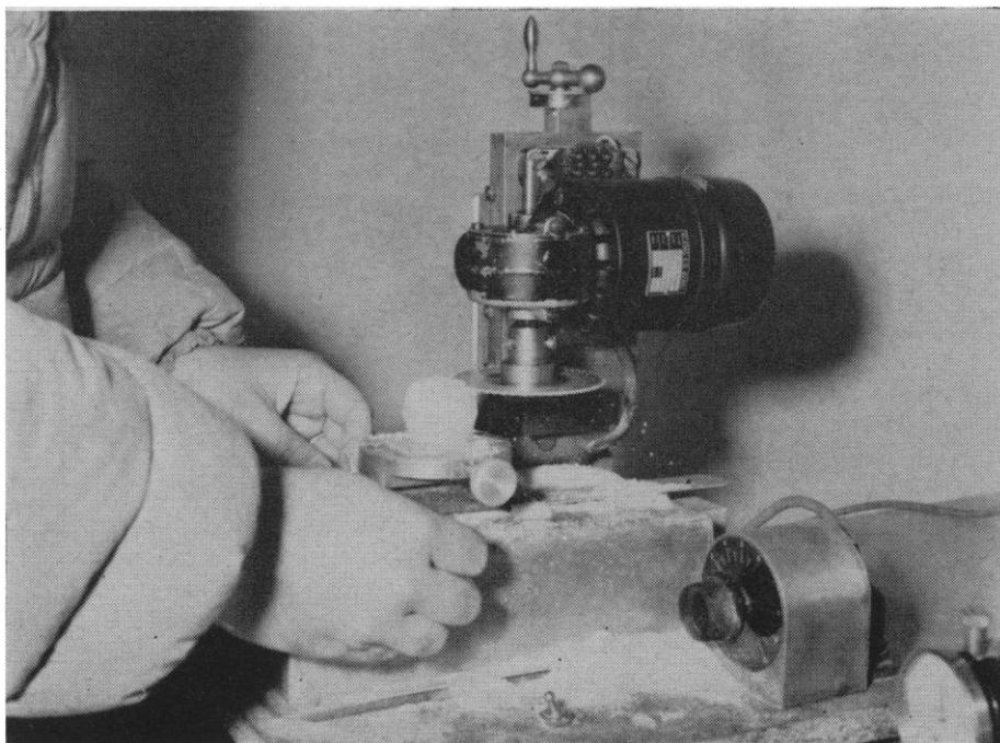
Fig. 2. Thin section saw.
