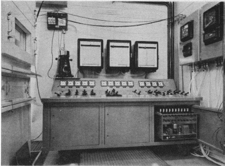
Fig. 9 (top). The measuring section of the tunnel, the control panel, the compensating recorders, and the regulating systems. Fig. 10 (right). The refrigerating compressor.
