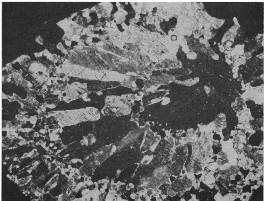
Fig. 4. Thin section of hailstone No. K 57.15, with polarized light (real length of the figure, 3.10 cm).
