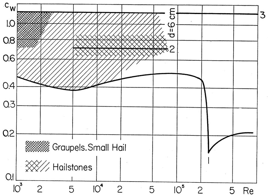
Fig. 6. Drag coefficient of graupels and hailstones as a function of the Reynolds number  $Re$ . Curve 1, values for smooth spheres; curve 2, values for ellipsoidal hailstones; curve 3, the drag coefficient for plates, giving an upper limit.
