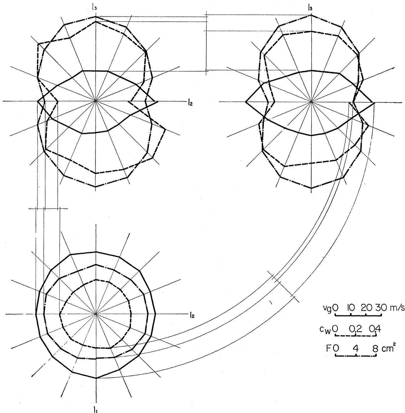
Fig. 5. Drag coefficient  $C_w$ , projection plane  $F$ , of hailstone No. K 47.24 in the direction of fall, and terminal velocity  $v$  in air, as a function of the position of free fall. Longest axes,  $l_3$ ; shortest axes,  $l_1$ ; medium axes,  $l_2$ .
