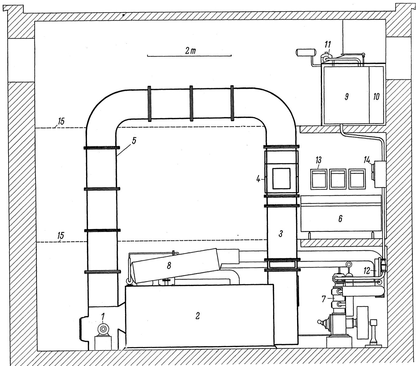
Fig. 8. The Swiss hail tunnel. (1) Blower; (2) section with refrigerating, heating, and filtering elements; (3) drop injection; (4) measuring place; (5) section for bringing the circulation back to the blower; (6) control panel; (7) refrigerating compressor; (8) liquid separator; (9) ammonia condenser; (10) alcohol-water cooler for cooling the refrigerating compressor; (11) oil separator; (12) motor valve; (13) compensating recorders; (14) regulating system for temperature; (15) floors.
