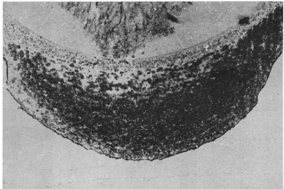
Fig. 11. Ice framework of an ice-water mixture, grown on an initial ice sphere with a diameter of 2.0 cm. Growing conditions: air temperature,  $-30^{\circ}\text{C}$ ; air velocity, 24 m/sec; free-water content,  $8.1 \text{ g/cm}^3$ ; resulting water content, 19 percent of the total deposit.
