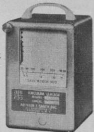
The smallest and simplest strip chart recorder on the market, it provides true rectilinear recording free from inconvenient distortion. Operating at one inch per hour, a 63-foot chart roll records for 31 days. A galvanometer pointer swings free for maximum accuracy, being clamped for marking briefly once every 2 seconds, generating a continuous line of many small dots. Scale length—2½". For portable use or panel mounting. 3¾" wide x 5½" high x 4¾" deep. Only \$193
