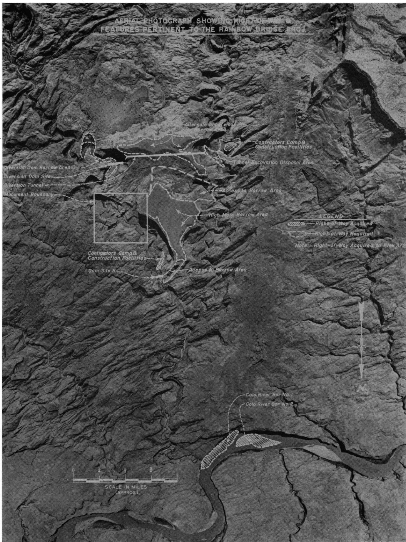
Fig. 2. A detailed aerial view of the national monument with superimposed outlines of construction planned to protect Rainbow Bridge from damage from the projected Glen Canyon Reservoir (Lake Powell). [U.S. Bureau of Reclamation]
