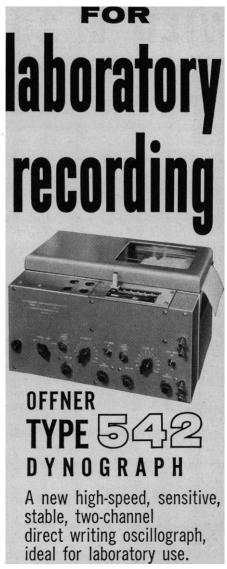
The OFFNER Type 542 Dynograph provides sensitivity—one MV d-c per mm; stability—with instant warm-up; rapid response—1.5 millisecond deflection time, —and large, easily read records—5 cm deflection with one percent linearity. Records everything from mechanical vibrations in the engineering lab to action potentials for the neurophysiologist.
