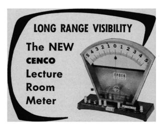
Now-a combination galvanometer, four-range voltmeter and four-range ammeter with figures and graduations on a large 17" scale that is plainly seen from both sides over any distance in the classroom. An accurate, versatile lecture meter with a modern, shielded movement. All parts and circuits clearly visible.
