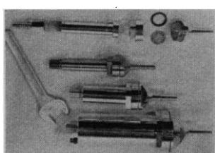
Vac-Pres Filters are bacteriological filters which may be used for vacuum or pressure filtration. These filters are available in 10 ml, 50 ml and 250 ml capacities. Other sizes upon request. The Vac-Pres Filters manufactured of brass with the interior silver plated and the exterior chrome plated. Stainless steel also available.
