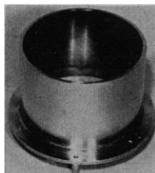
The Long Life Sieve is designed to allow the operator to replace the screen upon failure. The savings in cost of testing is realized when the cost of the replacement of the screen alone is compared with the cost of the replacement of the sieve screen unit as now practised. The frame of the sieve is constructed of chrome plated brass.
