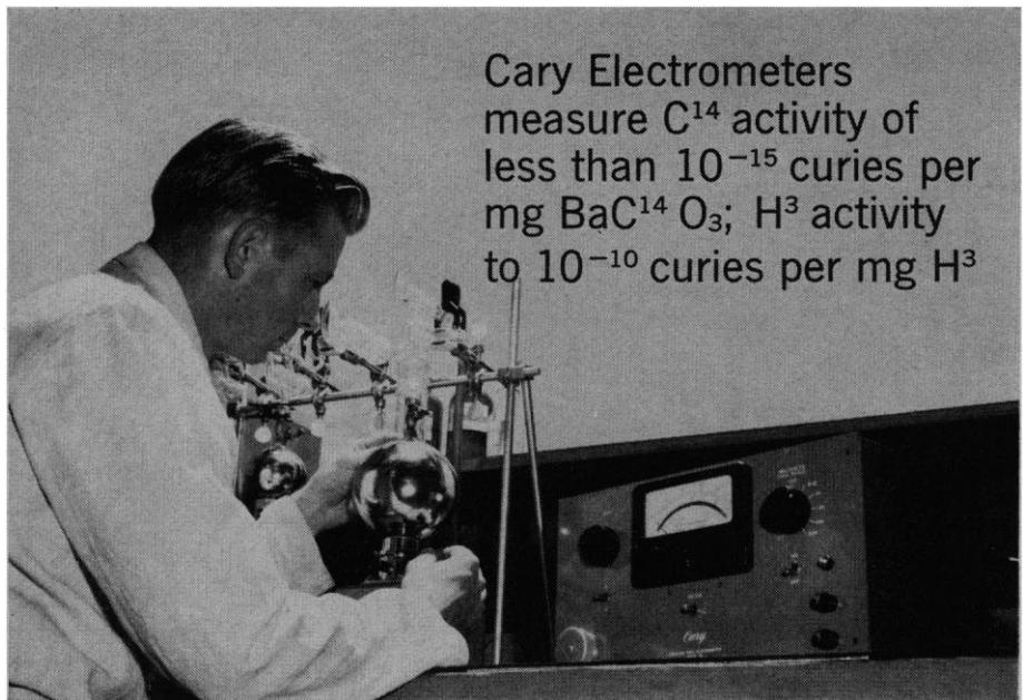
Cary Electrometers measure C<sup>14</sup> activity of less than 10<sup>-15</sup> curies per mg BaC<sup>14</sup>O<sub>3</sub>; H<sup>3</sup> activity to 10<sup>-10</sup> curies per mg H<sup>3</sup>
