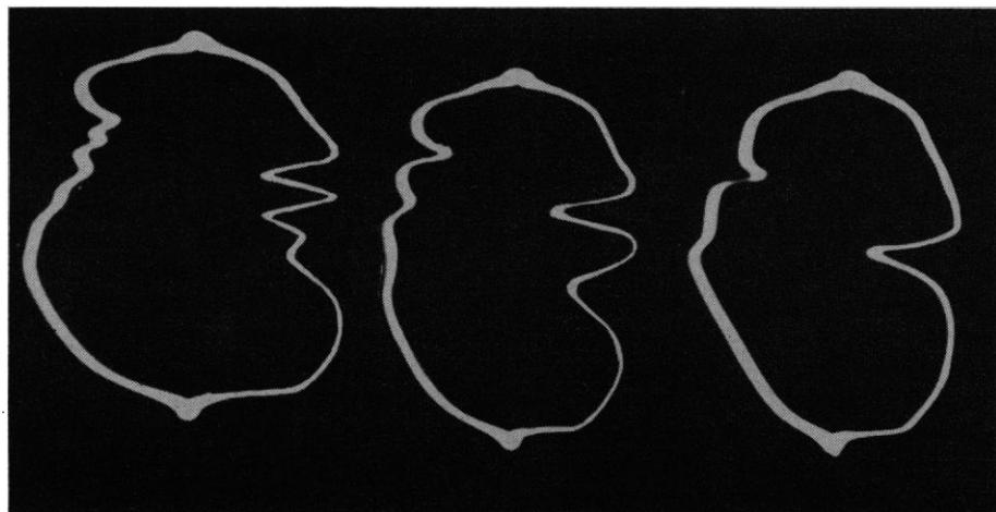
Fig. 26. Oscillographic diagram dE/dt = f(E) of o - and m -nitrophenol, apart and in mixture.
