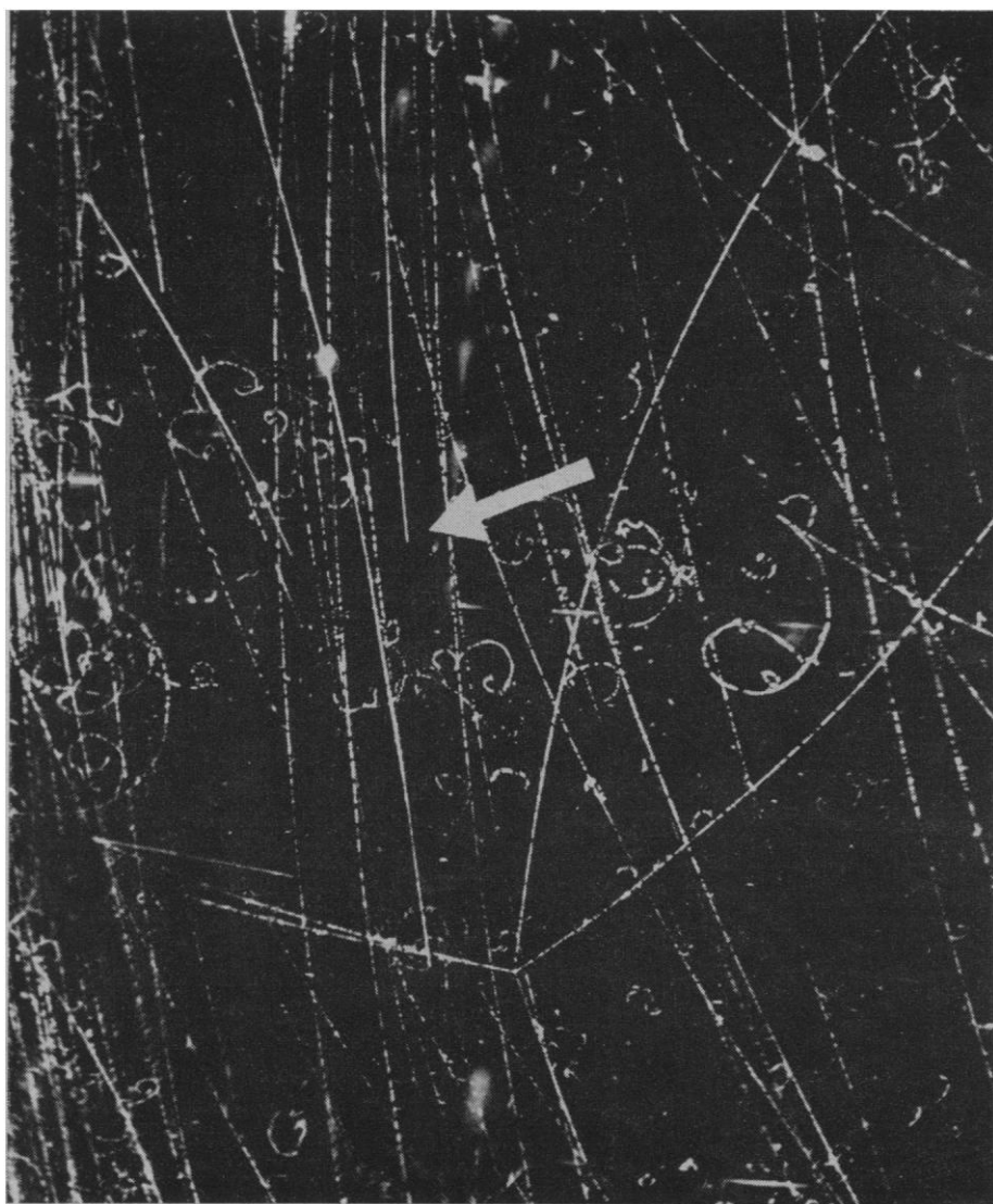
Fig. 1. An antiproton enters a propane bubble chamber, and at the point marked with the arrow undergoes charge exchange. The antineutron originates the annihilation star (directly below). Density of propane, 0.42 \text{ gm/cm}^3 . Real distance between charge exchange and origin of star, 9.5 cm. T_p at charge exchange, \sim 50 \text{ Mev} . [From Agnew et al. (6)]
