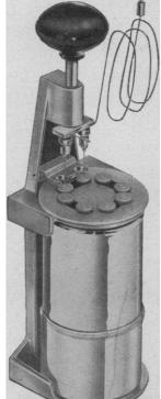
You can isolate exceedingly pure gas chromatograph fractions for supplemental analysis with this *single* instrument—the Hamilton Fraction Collector! It uses the "Freeze-Out" method of fraction collection, capturing the sample in a U tube on ultra pure silica sand chilled to liquid nitrogen temperatures... providing up to 98% plus recovery!
