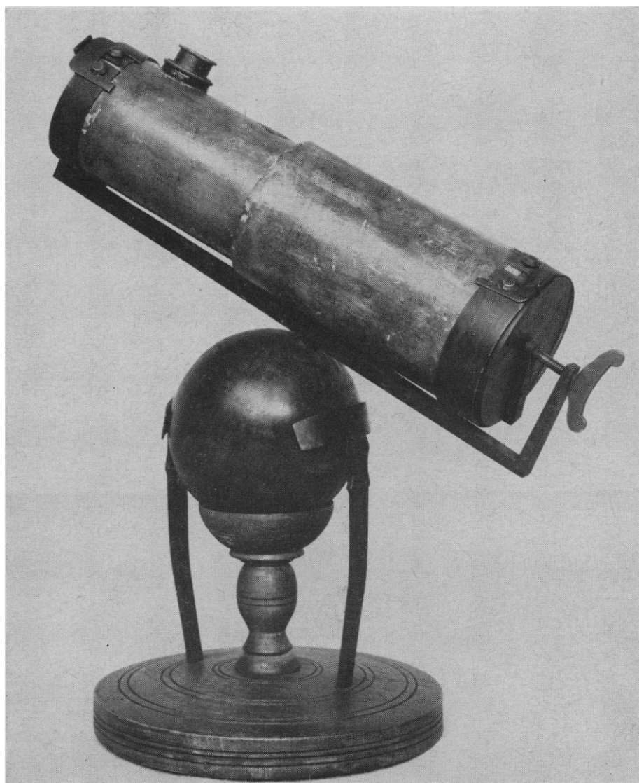
A facsimile of Newton's original reflecting telescope. [Science Museum, London]
