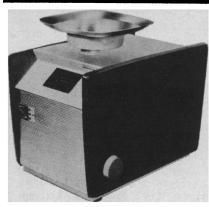
The only balance of its kind with full floating indicating mechanism for correct weighing regardless of off-level conditions. TOPPAN can be placed on any table and operated immediately without zeroing-in or leveling. Bright highly legible projection scale. No weights required. For weighing beyond optical range, just turn control lever to remove a substitution weight. The added capacity is indicated in window adjacent to projection scale.
