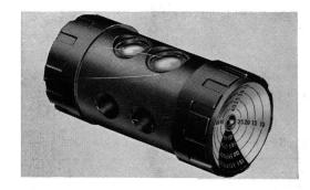
nifications are not required. Resultant magnifications can be varied from 10X to 40X by interchanging eyepieces, objectives or auxiliary lens attachments.
