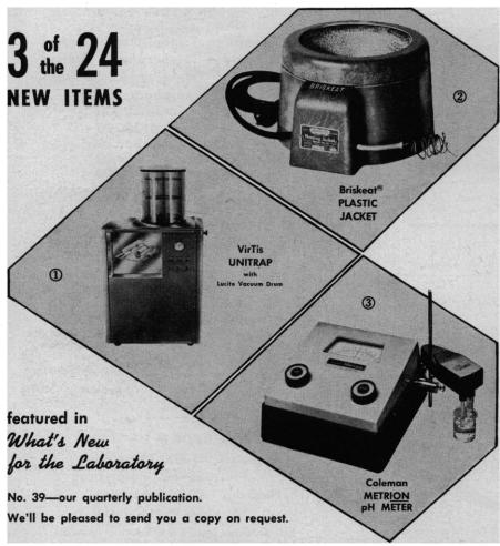
You can save up to six dollars a day by substituting the Unitrap for one requiring dry ice. This automatically-refrigerated cold trap is excellent for all freeze-drying procedures. Effluent capacity is three liters per dehydration. Easy to operate. Simply connect to a suitable vacuum pump after placing the required type of freeze-dryer on the top plate. For the complete Unitrap story, write for bulletin 14.
