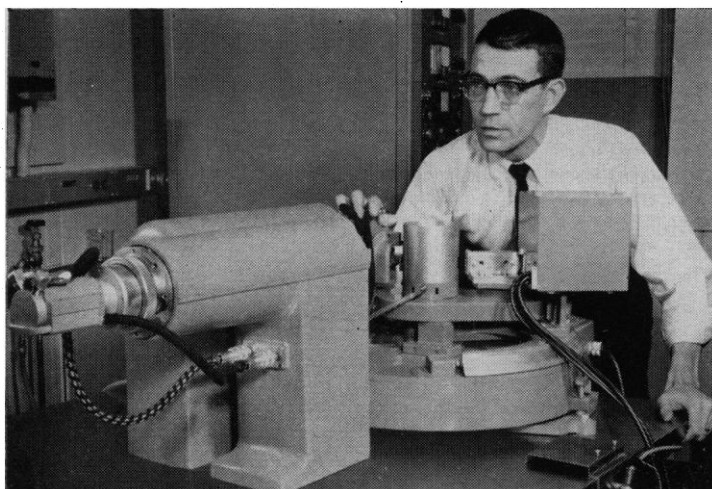
Chemist Jack Wright developed the use of this X-ray fluorescence machine for testing the concentration of preservatives in wood. Here he bombards a boring from a test telephone pole with X-rays.
