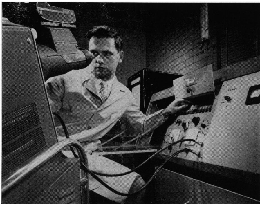
Roland Gohlke, Dow Chemical Company engineer, using Bendix Mass Spectrometer to identify compounds emerging from a gas chromatograph.
