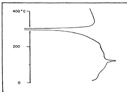
Fig. 2. Thermal record of the formation of galena by pyrosynthesis. The endothermic deflection to the right indicates the melting of sulfur, and the exothermic deflection to the left indicates the crystallization of galena.
