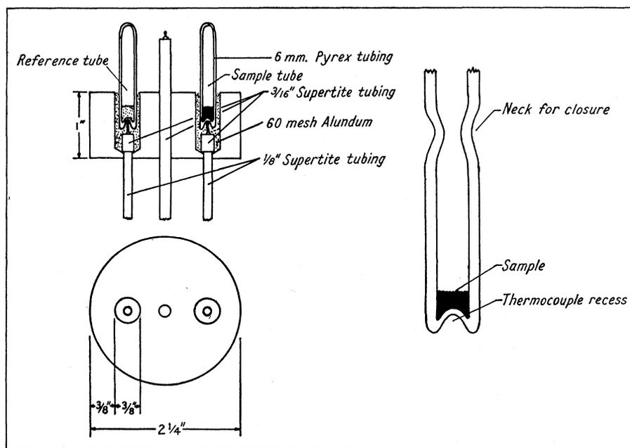
Fig. 1. Thermal head and detail of specimen vial.
