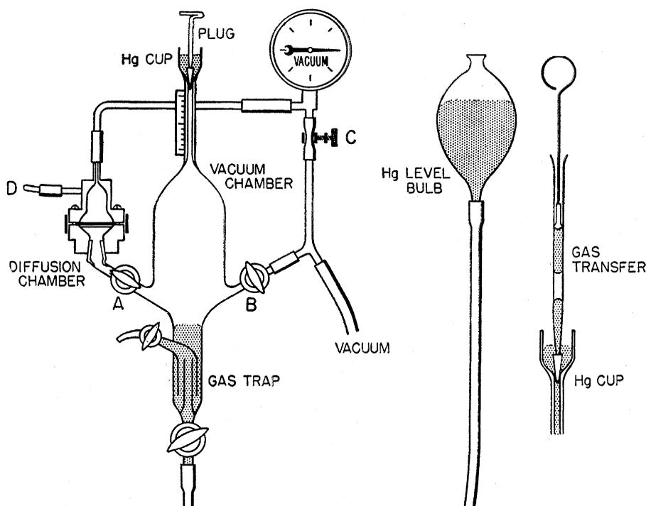
Fig. 1. Apparatus for steady-state diffusion.
