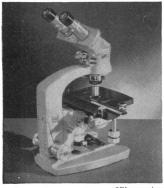
Optical path difference measurements can be made to an optimum accuracy of 1/300 wavelength. This unique ability to measure optical path thicknesses is in itself of great importance. But even more important, these measurements can be converted into a variety of quantitative information of great potential value. Water and protein content of a cell, for example, may be measured. Materials such as glass, plastics, emulsions, textiles can be examined.
