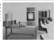
DIFFUSE REFLECTANCE ATTACH-MENT: A building-block utilization of the heated hohlraum technique, this attachment for the Perkin-Elmer Model 13 measures absolute spectral reflectance and emissivity in the range from 2 to 15 microns. KBr optics increase range to 20 microns.
