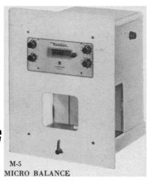
the M-5 micro balance with a precision of  $\pm 0.001\,\mathrm{mg}$
