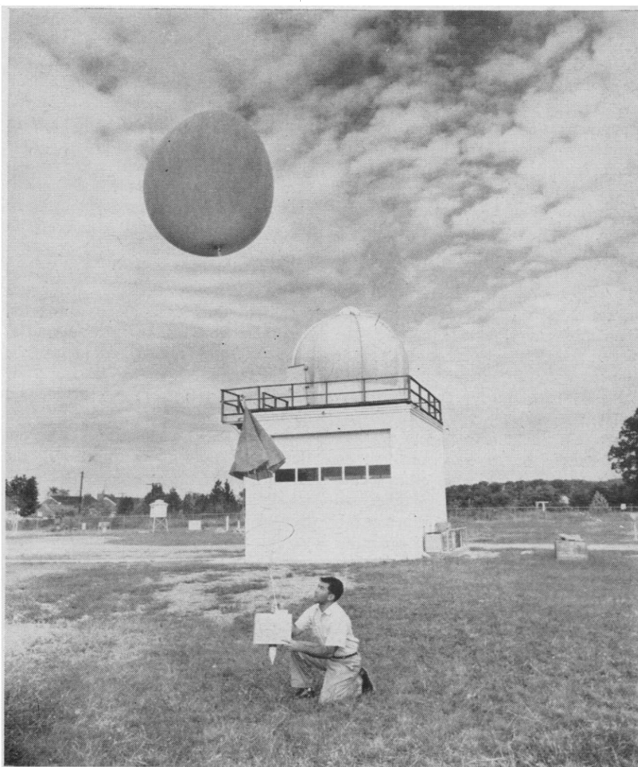
The U.S. Weather Bureau collects data for International Geophysical Cooperation-1959. Here a bureau observer holds an airborne rawinsonde assembly, consisting of a balloon, parachute, and rawinsonde transmitter. The Fiberglass dome in the background houses the rawinsonde receiver.
