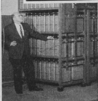
These energy-storage and discharge capacitors represent G-E custom design for optimum cost per joule in applications ranging from a few units to million-joule banks.
