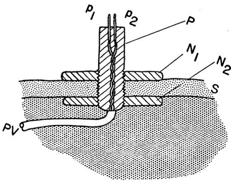
Fig. 11. Method of conveying the flow-meter leads through the animal's skin. *P*, threaded plug (cast from TDM); *P*<sub>1</sub> and *P*<sub>2</sub>, contact pins; *N*<sub>1</sub> and *N*<sub>2</sub>, nylon nuts; *S*, skin of the animal; *PV*, polyvinyl chloride tubing containing the lead wires.
