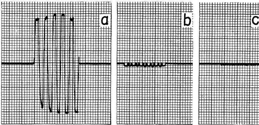
Fig. 9. Records showing the effectiveness of eliminating the transformer electromotive force in the external-magnet method by the use of a compensating coil and by means of a phase-sensitive detector (see text).
