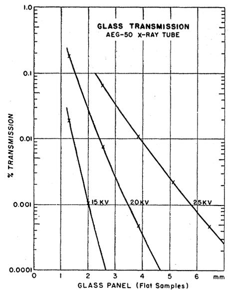
Fig. 4. Glass panel transmission curves.
