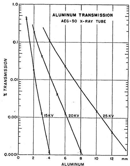
Fig. 5. Aluminum transmission curves.
