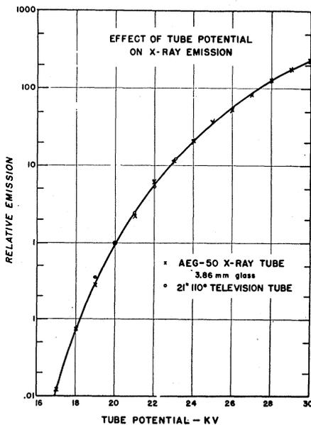
Fig. 2. Relative x-ray emission as a function of tube potential.
