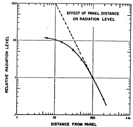
Fig. 3. Effect of panel distance on radiation level.
