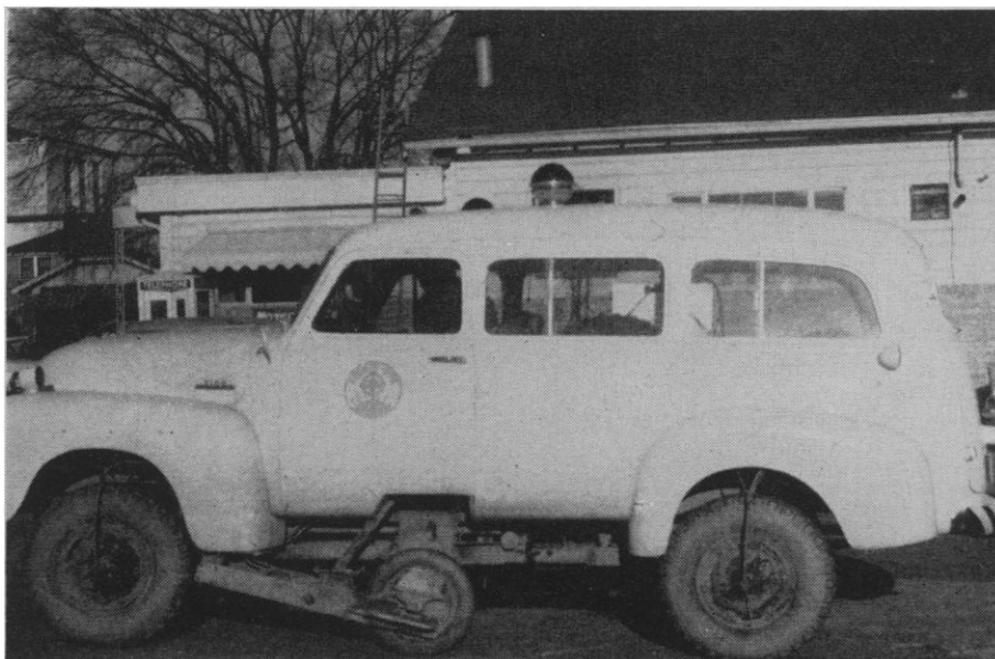
Fig. 11. The elevation meter. In this system, functions of the angle of slope and the distance traveled are integrated electronically, as the vehicle proceeds, to give height differences. The slope function is derived from the action of an electromagnetic field on a sensitive pendulum. [U.S. Geological Survey]
