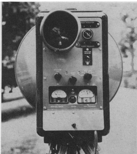
Fig. 9. The tellurometer. Distance measurement with this instrument depends on the known velocity of radio waves. [U.S. Geological Survey]
