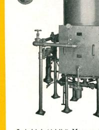
**Typical Industrial Unit:** Mass production steam heated Still with automatic controls. 50 to 500 gallons per hour capacity.
