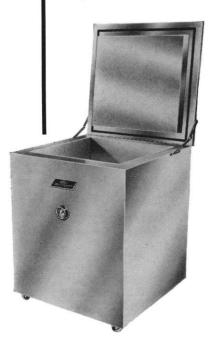
Capacity 400 lbs.; on swivel casters. Of double-wall plywood construction finished inside and out with white epoxy enamel and with 2-inch Freon-foamed-in-place urethane insulation. The use of cellular foamed plastic (Fluorofoam) containing low thermal conductivity Freon gas makes this chest superior to cabinets insulated with cork or glass wool, and also results in lighter weight.
