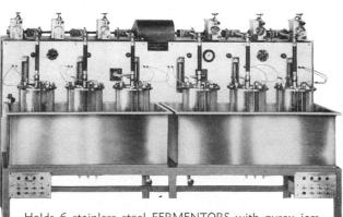
Holds 6 stainless steel FERMENTORS with pyrex jars of capacities 5, 7.5 or 14 liters each; removable for autoclaving. Leak-proof, non-freezing, ball-bearing agitator housings. Cool, quiet, continuous performance.
