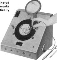
A mere touch of each colony with an electric probe actuates an electromagnetic counter and leaves an identifying puncture in the agar. When puncturing is not feasible, a marking pen may be used which marks the glass plate as it counts. Complete with push button counter, automatic reset to zero and magnifying viewer.
