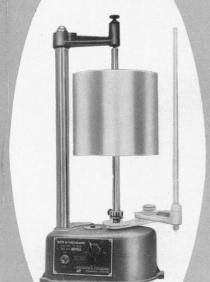
A motor driven recording drum that is very suitable for students' use and also for general experimental work.
