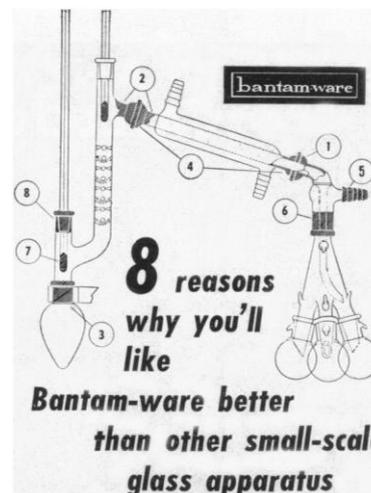
**1. NO POCKETS** to catch the product. Ball-and-socket connections let product flow straight through without hold-up.
