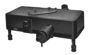
with exchangeable prisms for the visible, ultraviolet, infrared from 200 millimicrons to 20 microns
