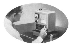
A major advance in weighing instrumentation combining a novel application of physical principles with modern engineering design, the Cahn Electrobalance is unaffected by vibration, or temperature change. You can use it anywhere, and depend on it.
