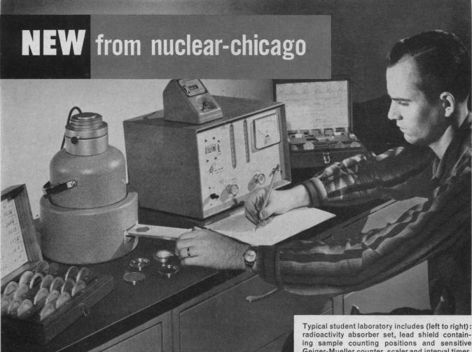
radioactivity absorber set, lead shield containing sample counting positions and sensitive Geiger-Mueller counter, scaler and interval timer, and radioactivity standards, sources and sample preparation kit.
