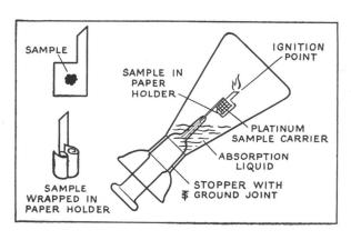
with free-flowing oxygen. The paper tail is then ignited; the stopper with flaming sample is seated in the flask and flask then inverted at an angle. The catalytic combustion proceeds at high temperatures and the combustion products are absorbed in the liquid, which forms a seal around the stopper. After cooling, the inside surfaces of the flask and stopper are thoroughly rinsed. *Titrations can then be made directly in the flask*.
